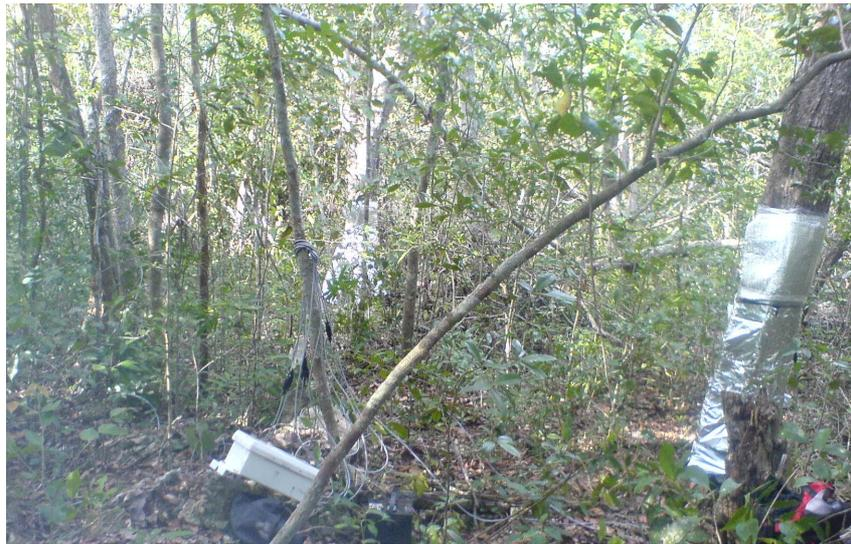
**Figure 4-27:** A photograph from site 4 showing some of the sample trees (covered with insulation and aluminum foil) and the datalogger (in the white box).
