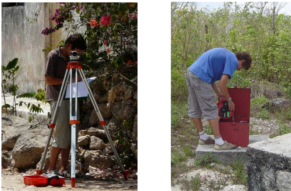
Figure 14: Picture of leveling (left) and water level measurements (right)
