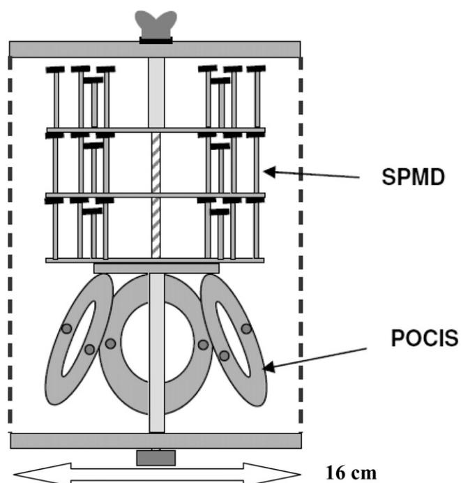
**Fig. 2.** Configuration of stainless steel cage used to deploy SPMD ( $n = 3$ ) and POCIS ( $n = 3$ ) passive samplers in cave systems in the study area.
